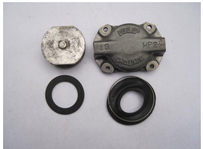
Cylinder disassembled. Piston, cylinder body, piston seal and dust cover.
